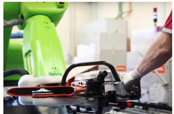
Figure 7. Cobots holding STIHL cut-off machine for operators to inspect Source: IFR (2018a)
